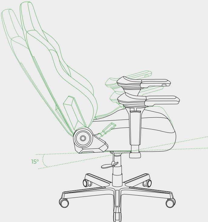
Pull out the right lever to enable the rocking function
