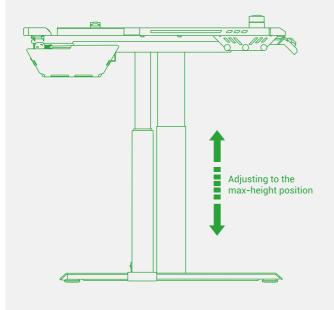
If your memory height exceeds the maximum (minimum) height limits, the setting will be invalid. You must reset the memory position
